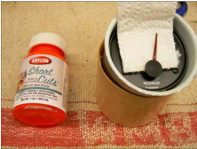
Did you know that you can synchronize your voltmeter to better reflect the true voltage coming from the battery? The BMW voltmeter displays about 1/2 to 1 volt less than the battery output due to voltage drops and how it's wired in the system. Since we have it apart why not adjust it to show true battery voltage? This transitions the voltmeter from an indicator to a much more accurate instrument.
