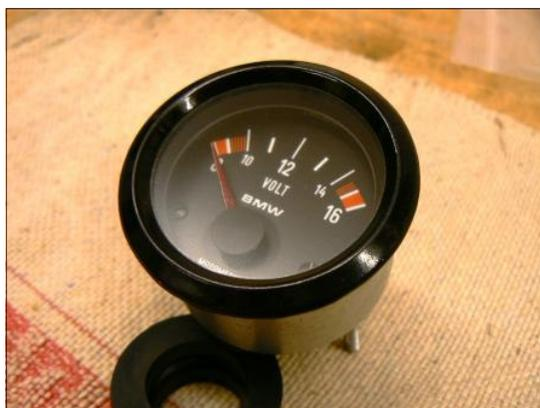
The protective lid is 'rolled' over the cylinder to form a seal and keep water and dirt from entering the front. To open the unit up we turn it over and use a small flat bladed screwdriver to gently separate the cover from the cylinder.
