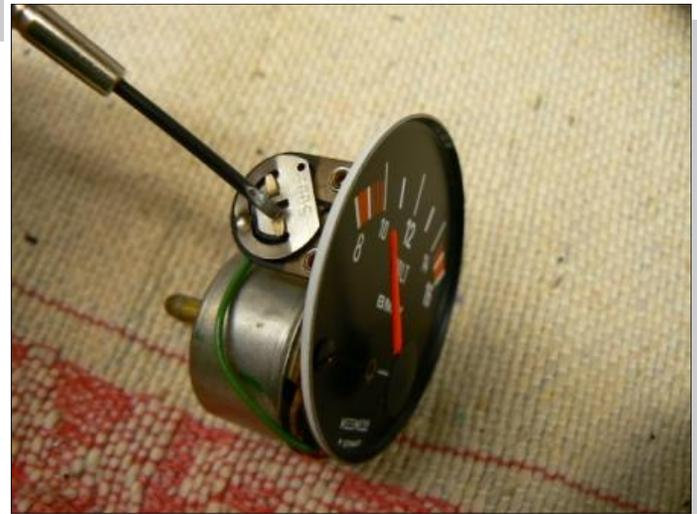
3,000 rpm and then compare settings. The battery voltage should read around 14v. Then, just rotate the dial on the BMW voltmeter showing the same voltage. It's that easy.
