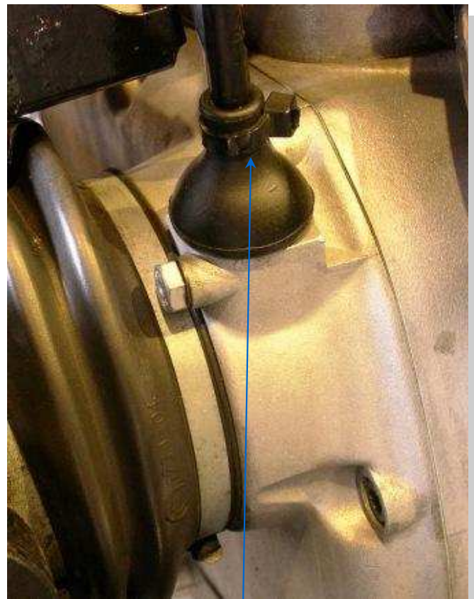
A simple wire tie will do the job, keeping water and dirt out. It also helps to fill the boot with some grease. Ed.
